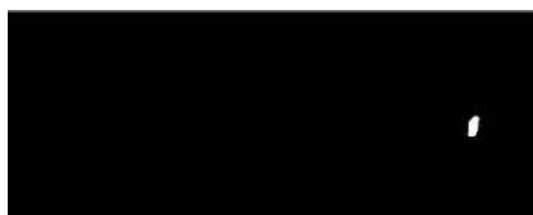
Fig. 3 - No more direct beam. Only Cu K \alpha contributes to this intense small spot.
