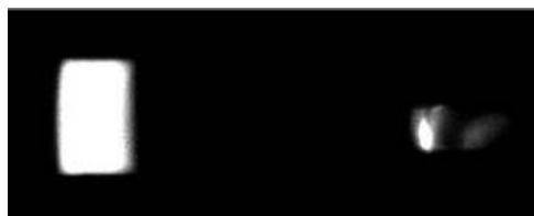
Fig. 2 - Remaining direct beam and medium energy. Reflected beam Cu K \beta appearing on the right.
