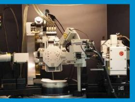
Fig. 1 : Bruker D8 X-ray diffractometer equipped with FOX2D optics.
