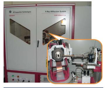
GE Inspection Technologies X-Ray Diffraction System Seifert XRD 3003 PTS
