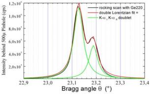
Graph 1: Rocking scan characterisation of the mirror beam (500 µm exit) with a Ge220 crystal on the sample goniometer.
