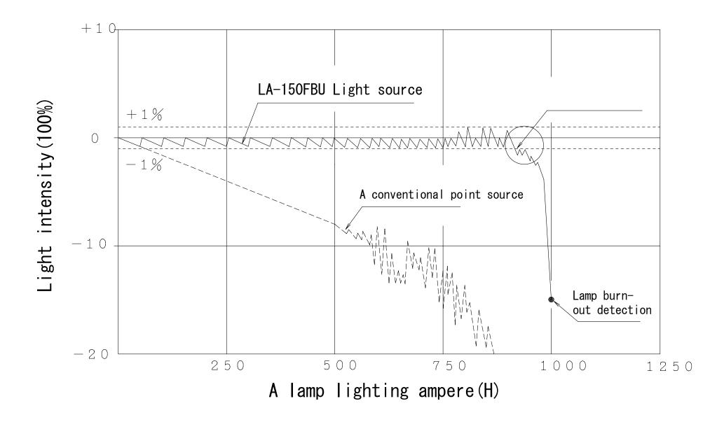
The figure is a luminous energy state of a conventional point source apparatus, and a new point source apparatus.
