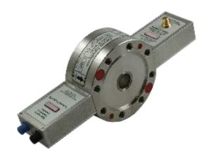
**Turbo-ICT** is mounted directly on the beam line UHV compatible to  $10^{-10}$  mbar Ceramic gap vacuum-brazed over Kovar transitions Material AISI-304
