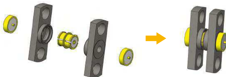
(Installation of SMP Connectors)
