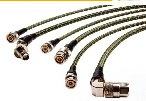
GigaLane GLA & GULA cable assemblies have been developed and produced for aircraft and cover broad frequency ranges from DC to 18 GHz. These high qualities, low loss cable assemblies deliver a low VSWR of 1.35:1, feature a self-locking connector and are protected by a Nomex and Kevlar jacket, which offers abrasion resistance.
